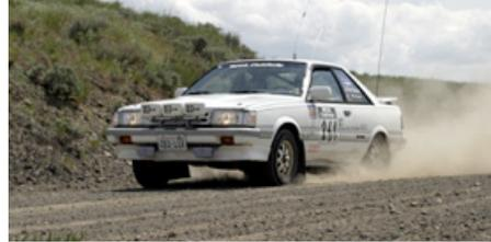
1987 Subaru RX Coupe GL 3-door 1.8 liter Turbo (EA82T) 5-speed dual-range transmission, Bilstein 40mm coil-over suspension
